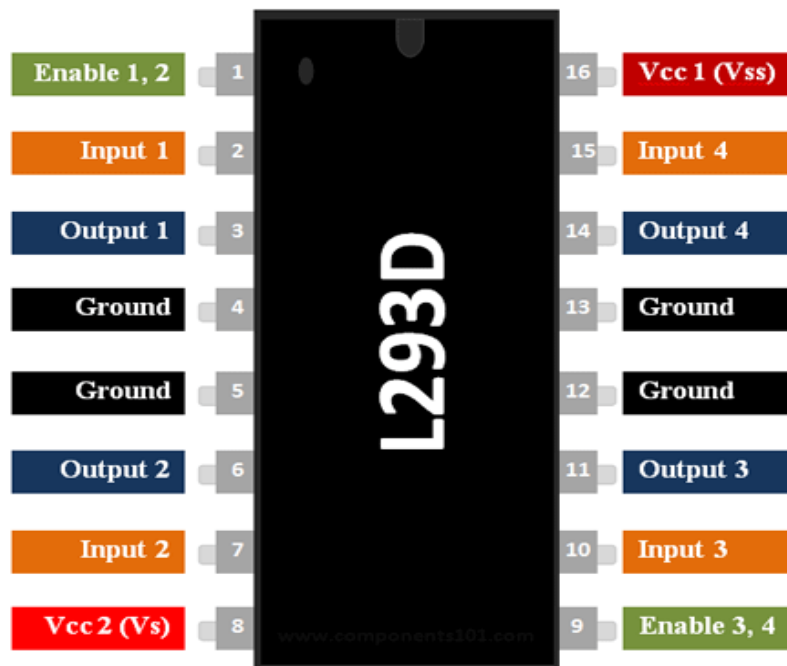
Fig 5.16: Pin Details of L293D IC
