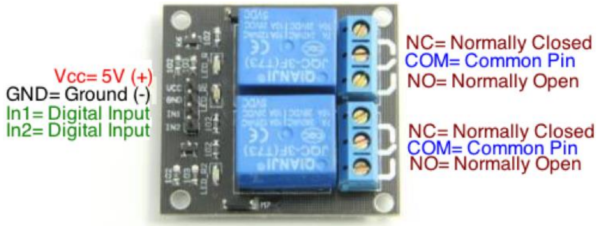
Fig 5.20: Pin Description of Electromagnetic Relays
